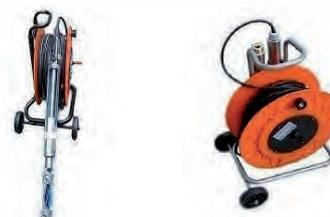
P/S Wave Borehole Energy Source Borehole Deviation Probe
