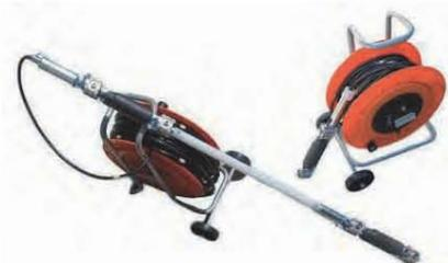
3D/5D - 3D Twin Borehole Geophone
