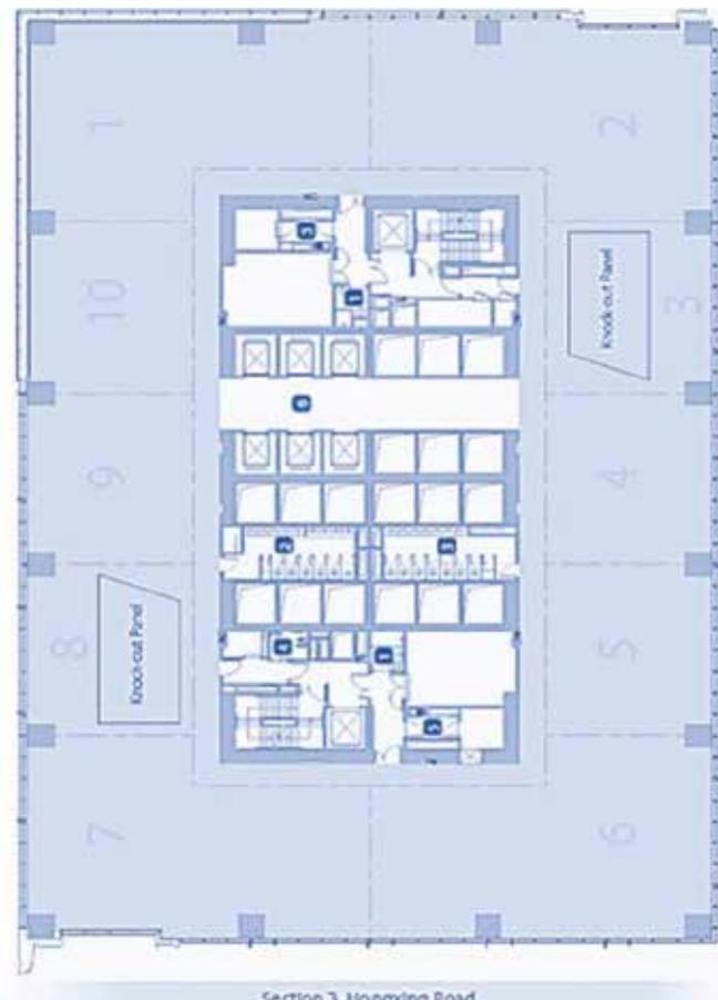
Fig. 3 | IFS Tower (Office building, 250 m structural height / 50-floors / floor dimension: 65x44 m – +/- 2900 m<sup>2</sup> average gross area per floor), Chengdu, China
