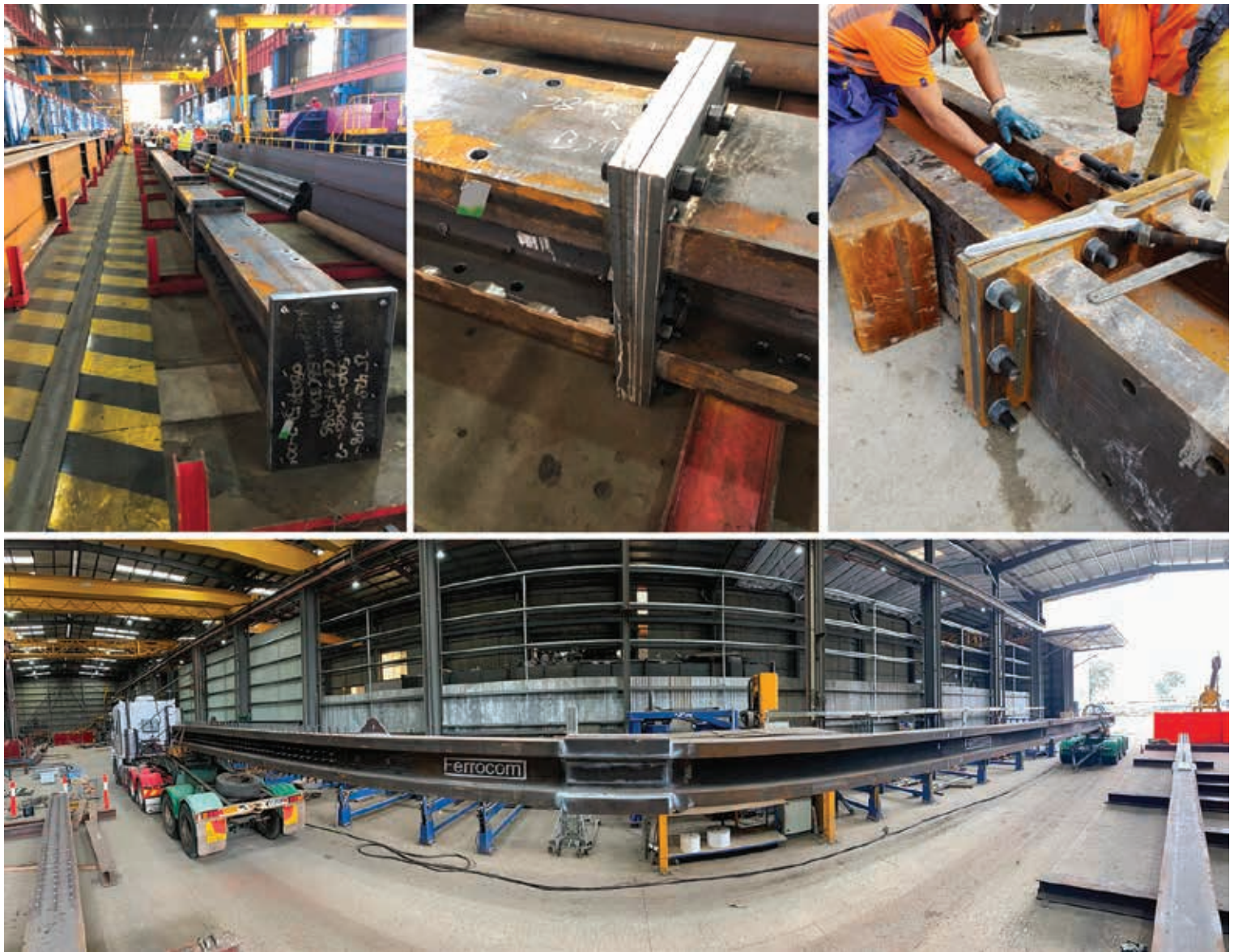
Fig. 10 | Example of a bolted end-plate-connection (up); example of a contact surface connection with small welded cover plates to ensure bending moment resistance (down)
