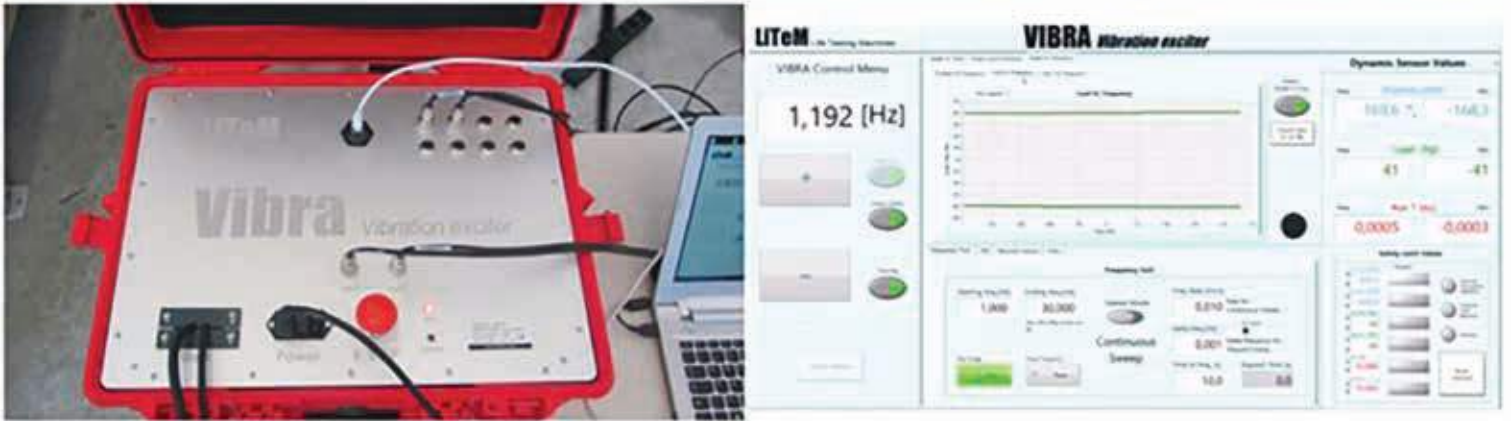
Fig. 6 | Vibrodina lineare VIBRA 9001, controller e software – Litem - life testing machine
